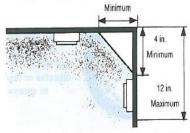
The ceiling is the best mounting locationat least four inches away from any walls. If detectors are mounted on the wall, keep them away from corners and at least 4 inches, but no more than 12 inches, from the ceiling to the bottoms of the detector.
